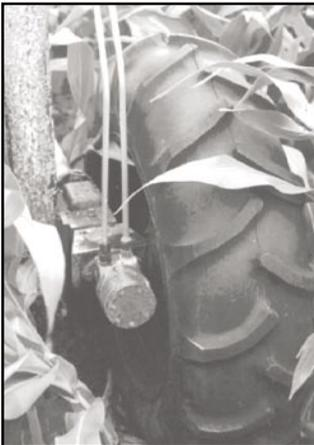
This unique worm drive design features an automatic built-in brake that will prevent the system from coasting. One hydraulic motor is utilized per tower. Oil is supplied to the motor by high pressure steel lines and fittings. A variable flow control valve regulates direction, speed and, when required, provides an optional safety for misalignment.
