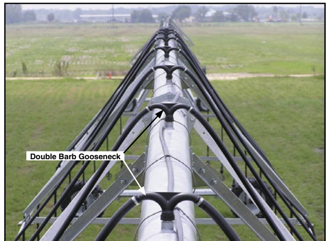
The Double Gooseneck makes installation of additional outlets easier.
