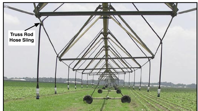
The Truss Rod Hose Sling holds drops in the desired position along the truss rod.
